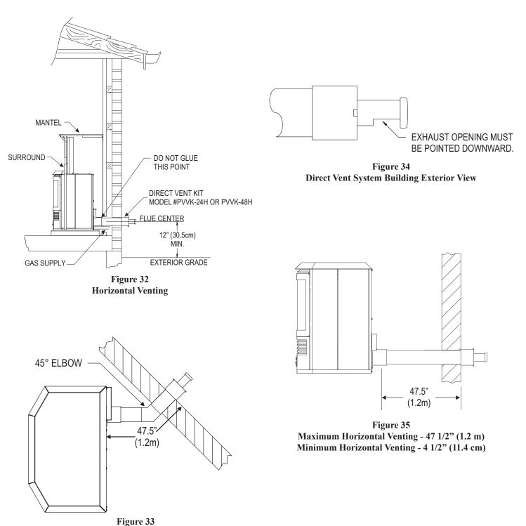
Horizontal Venting Maximum 47.5" (1.2 m) with a 3", 45° elbow 3", 45° elbow can be purchased from a local hardware store
